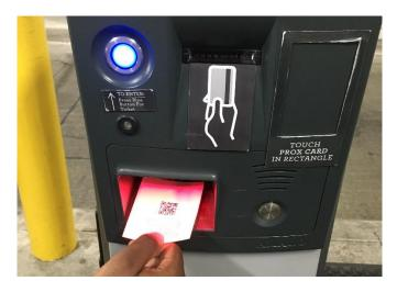
**Step 4:** Machine will process barcode and/or QR code and if approved, will open the gate for exit. If NOT APPROVED, vehicle will be required to pay the maximum daily rate.
