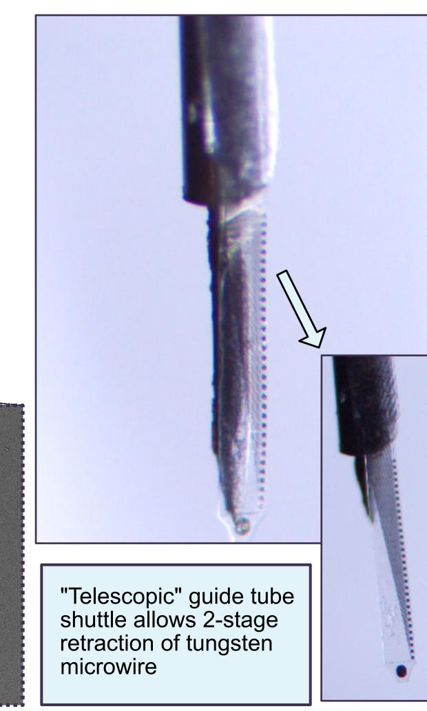
State-of-the-art, high-density penetrating electrodes enable probing of neural circuitry. However, their stiffness fails to accommodate the brain's natural oscillations caused by respiration and cardiac rhythm.
