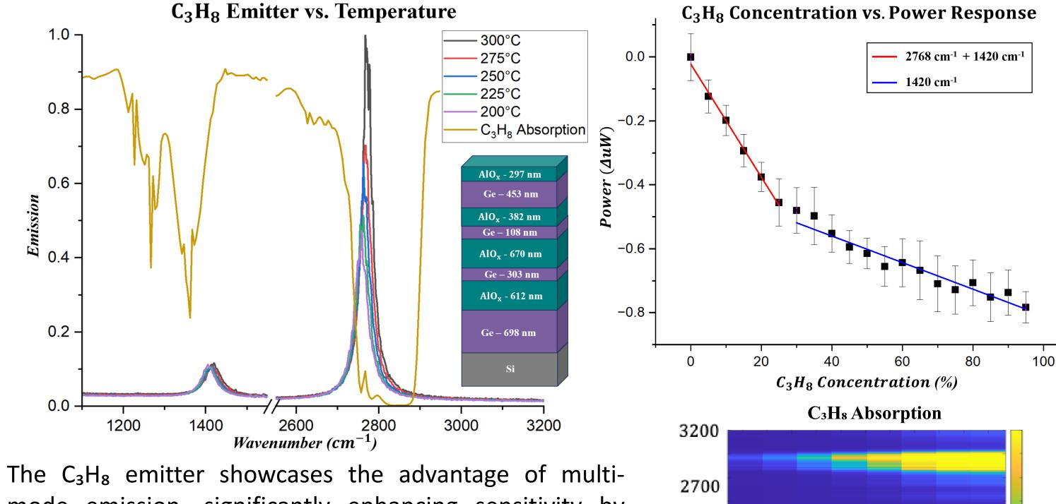
mode emission, significantly enhancing sensitivity by targeting multiple absorption bands simultaneously. This approach results in much higher combined absorption compared to NDIR sensors, which are limited to singleband emission<sup>11</sup>. By leveraging multiple vibrational modes, the propane emitter optimizes sensitivity and surpasses the limitations of traditional NDIR systems.<sup>8</sup>
