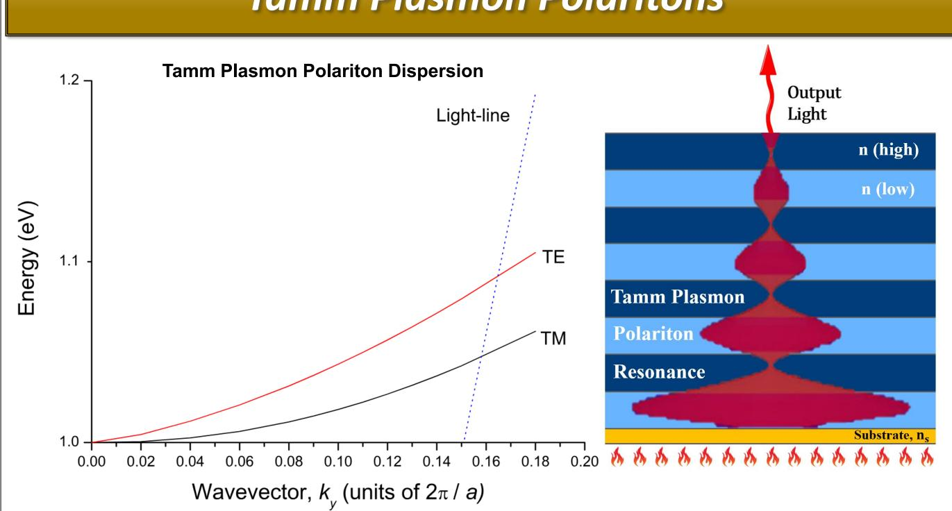
Tamm plasmon polaritons (TPPs) occur when a SPP resonance is coupled to a wavelength matching photonic band gap of a photonic crystal. The dispersion of a TPP lies within the light cone, allowing it to be excited by both TM and TE modes without the use of prisms or gratings.<sup>4</sup> This results in deep penetration length and optimized emission.
