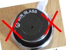
Eyepiece Solar Filter: After unfiltered sunlight is focused onto an eyepiece solar filter, the intense heat will cause the filter to crack and let through unfiltered sunlight. Credit: Stephen Tonkin
