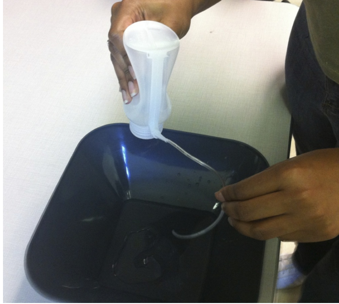
Figure 5. Hands-on demonstration with air being pushed through the hose by squeezing the bottle upside down.
