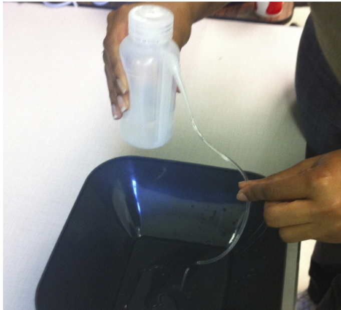
Figure 6. Hands-on demonstration with water being pushed through the hose by squeezing the bottle right side up.
