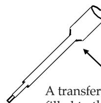
A transfer pipette, filled to the base of the bulb (as indicated by the arrow), holds about one milliliter of liquid (1.0 mL).
