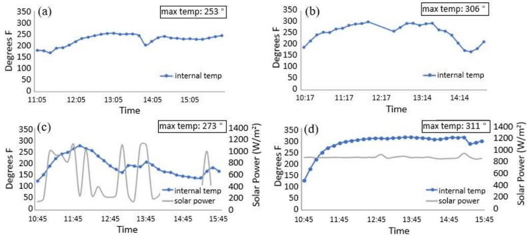
**Figure 2.** Four of the oven’s significant temperature performances. (a) oven’s highest internal temperature in Phase 1, (b) the oven’s performance immediately following usability and efficiency improvements, (c) oven’s internal temperature on a partly cloudy day, (d) oven’s internal temperature on a cloudless day, which illustrates the effect of solar energy on the oven temperature growth.
