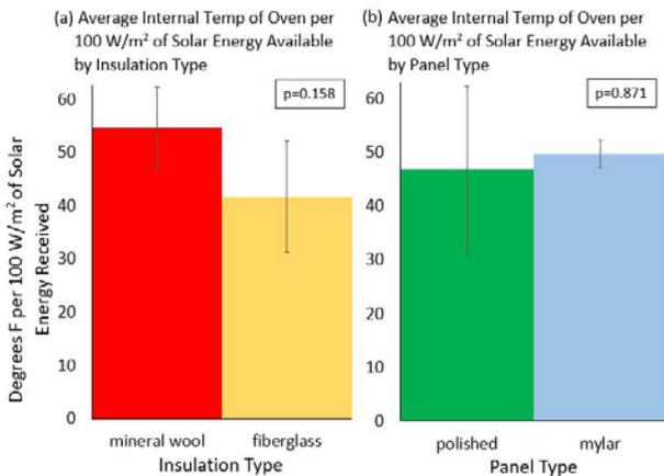
**Figure 3.** Two types of insulation were tested alongside two types of panels on the oven to determine whether any one material would result in a significantly better temperature output. Temperatures achieved by the oven were standardized according to solar energy input. Average internal temperature of oven in terms of solar energy input by (a) insulation type and (b) panel type.
