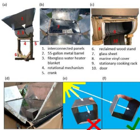
**Figure 1.** The oven's main design aspects and alignment tutorial. (a) full-size oven model, (b) top view of oven cooking chamber and attached panels, (c) side view of cooking chamber with door open, (d) the solar alignment cube in correct positioning on the oven, (e) the solar alignment cube improperly aligned with the sun, (f) the solar alignment cube properly aligned with the sun.
