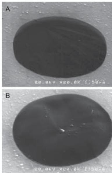
**Figure 2.** Scanning electron microscopy of graphene before (A) and after (B) electron transmission experiment. Carbon build up is noticeable in 'B'.
