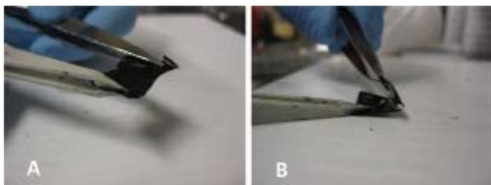
**Figure 2.** Photographs showing PEPDECS-liberated CNT films. (A) shows the relatively intact shape of the film and (B) demonstrates the flexibility and stability of the films. The tear seen on the edge of the film in (B) was inflicted during the removal of the film from the water in which PEPDECS was conducted.
