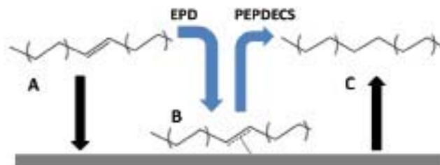
**Figure 3.** Electrochemical deposition scheme for EPD and PEPDECS. (A) During EPD, CNTs reach the positive electrode and are linked onto it by a double bond located in the organic chain of the surfactant. (B) During PEPDECS, hydrogen generated from electrolysis of water reacts with the complex [(surfactant double bond)-(steel)], reducing the double bond and (C) releasing the CNTs.
