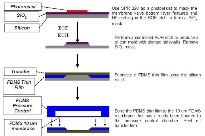
**Figure 2.** The process for fabricating the devices. It is important to note that the membrane was spin-coated on inactive plastic film while the PDMS thin film lower pieces were fabricated using a coated plastic transfer film.
