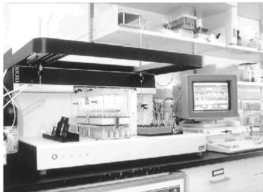
Figure 2. A now dated photograph of the 40-array apparatus interfaced to the x,y,z robot used for liquid delivery (September 1993).
