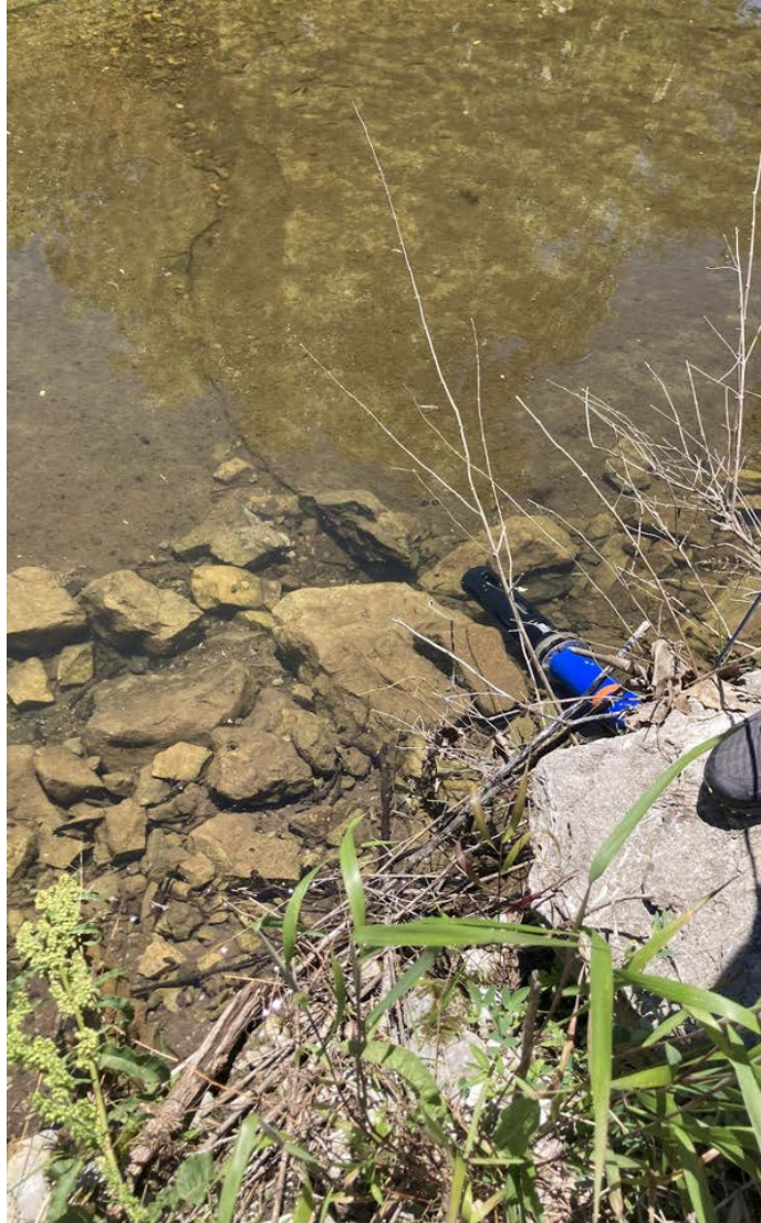
Figure S3. The EXO2 sonde placed in the water at 35.9515437 N, -87.015628 E, off of the bank the East Fork Creek for data collection, taken 06/03/22. The sensor is completely submerged in the water, but secured to the bank using multiple cables.
