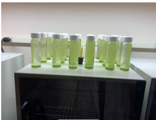
Figure S1. Set-up for the 24 hours hydrogen generation period. Arranged vials in a 6x4 rectangle, each row of 6 being one category, with each vial labeled appropriately. 24 hours was chosen both for practicality as well as previous literature indicating this was when hydrogen production peaked [5].
