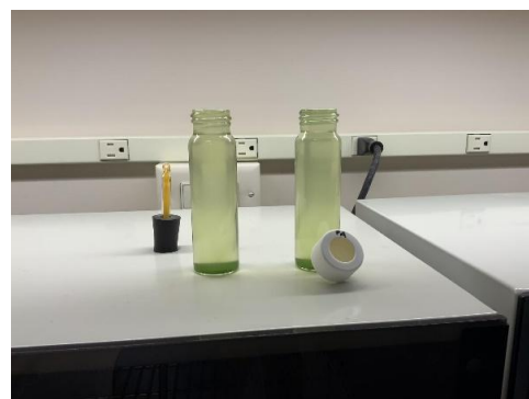
Figure 2. Titration process. A color comparison between a titrated vial (right) and un-titrated vial (left). Done directly under bright light to ensure accuracy in color comparison, though the difference became slim at times.
