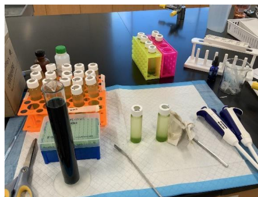
Figure 1. The titration process setup with reagent in a graduated cylinder and micropipettes used for adding reagent dropwise located on the table.
