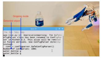
Figure 4. Hand recognizing a Pet bottle using AI program.
