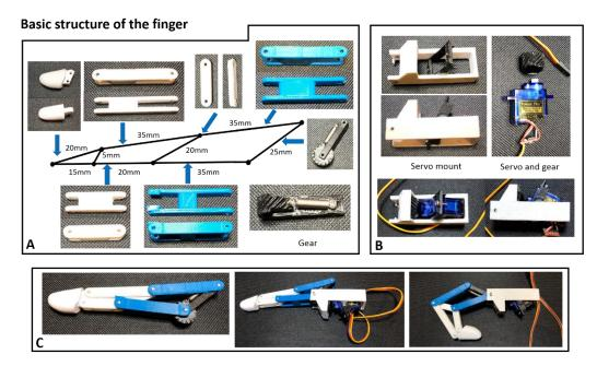
Figure 2. Basic information about each finger with underactuated mechanism. (A) The finger joints and their respective lengths. (B) The way that the servo is mounted to the finger. (C) Overview of the whole finger and how it bends.
