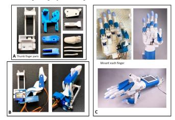
Figure 1. Overview of the prosthetic with AI. (A) Basic components need to build a thumb. Overview of the (B) built thumb and (C) whole prosthetic.
