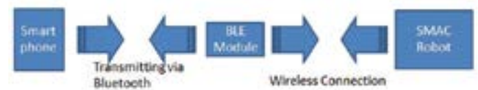
Figure S1. Diagram of the Bluetooth module from Anaren Atmosphere is being implemented in the connection between a Smart phone’s application to the SMAC robot.
