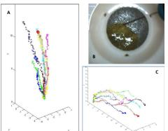
**Figure 2**. Membrane peeling results: **A**. One successful peeling; **B**. Gripper tip motion when peeling straight up; **C**. Gripper tip motion when peeling up and roll over.
