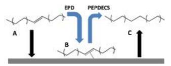
**Figure 3.** Electrochemical deposition scheme for EPD and PEPDECS. (A) During EPD, CNTs reach the positive electrode and are linked onto it by a double bond located in the organic chain of the surfactant. (B) During PEPDECS, hydrogen generated from electrolysis of water reacts with the complex [(surfactant double bond)-(steel)], reducing the double bond and (C) releasing the CNTs.
