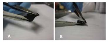
**Figure 2**. Photographs showing PEPDECS-liberated CNT films. (A) shows the relatively intact shape of the film and (B) demonstrates the flexibility and stability of the films. The tear seen on the edge of the film in (B) was inflicted during the removal of the film from the water in which PEPDECS was conducted.
