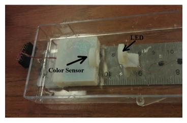
Figure 1 shows the testing apparatus that was used to assess the color sensor.
