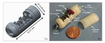
**Figure 2** shows the configuration of the capsule protocol. (2A) Design of the capsule shell as created on Creo Parametric 2.0. (2B) Structural view of the physical capsule prototype.
