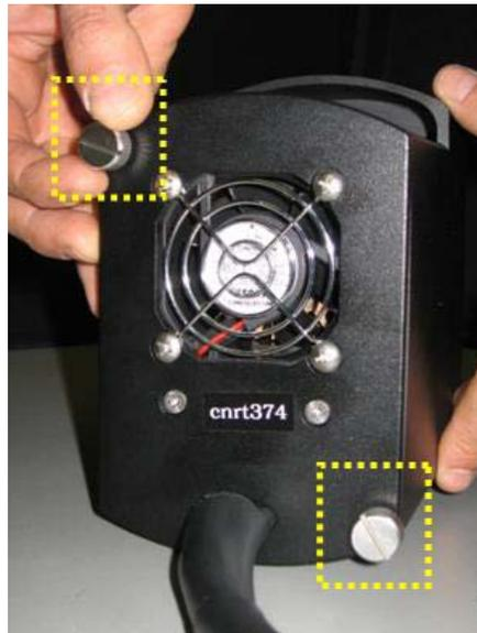
12. Place the open end of the lamp housing over the flange on the DeltaVision and tighten the three hex screws as shown.
