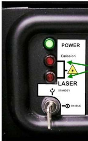
Emission indicator lights are ON when interlock is closed.
