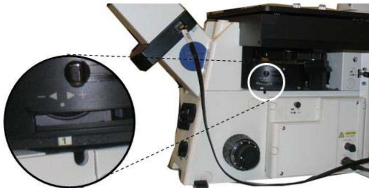
Figure 3.5 Polychroic filter wheel control
