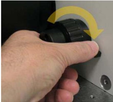
11. Lower the objective by turning the Coarse Z Focus knob away from you when facing the knob (clockwise on the right-side knob).
