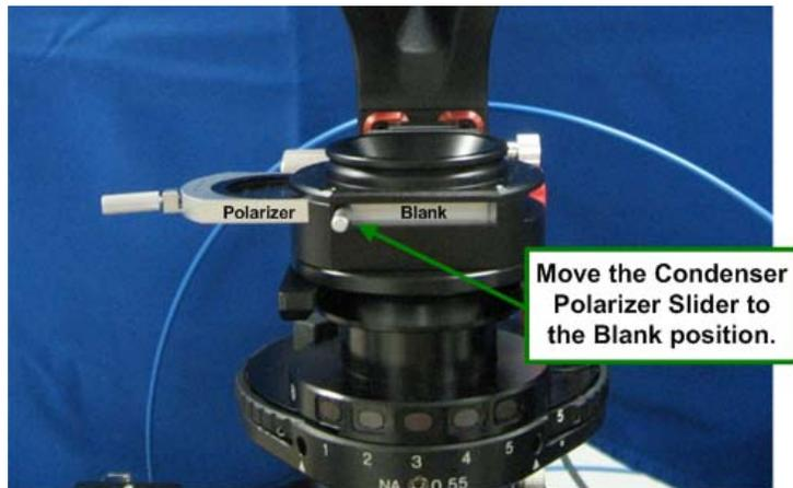
2. Rotate the Condenser Prism Turret to a blank position.
