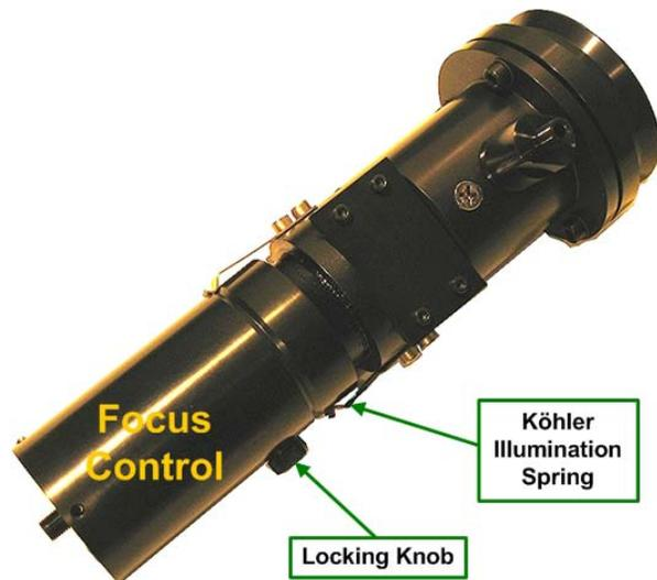
The FOM in the Köhler Illumination position, the Fiber Optic Module is pushed in so that the Köhler Illumination Spring is in the groove.
