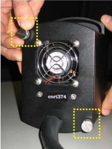
5. Gently slide the internal lamp mechanism from the lamp housing.
