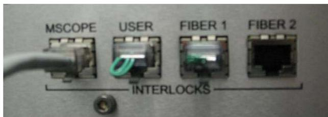
For the lasers to operate, all of the following safety devices must be set as follows:
