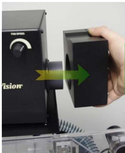
The filter box is held in place by magnets. Simply pull out to remove.
