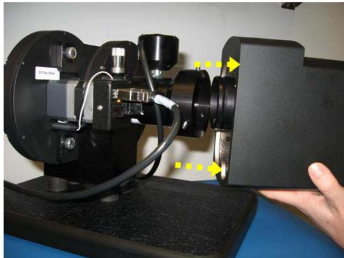
4. Loosen the two thumb screws on the opposite end of the xenon lamp housing.
