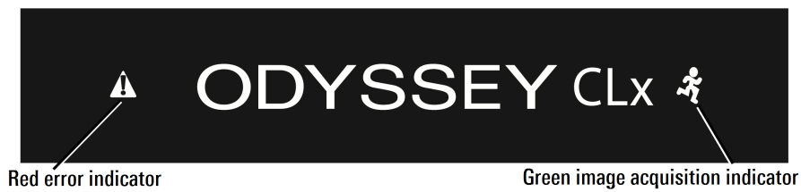
Figure 2-2. Location of the green image acquisition light and red error light.
