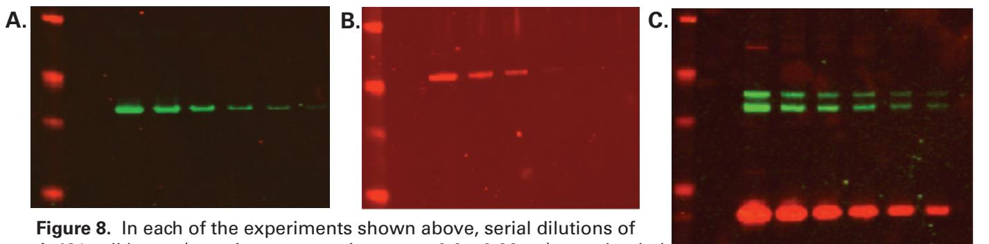
**Figure 8.** In each of the experiments shown above, serial dilutions of A-431 cell lysate (protein concentration range 2.0 – 0.06 µg) were loaded onto polyacrylamide protein gels, electrophoresed and transferred to membrane using the iBlot Dry Blotting System (Invitrogen). Detection was performed using IRDye labeled secondary antibodies and the Odyssey Infrared Imager. (A) ERK2 (B) βTubulin (C) Cofilin (red, 700 channel) and phospho ERK (green, 800 channel).
