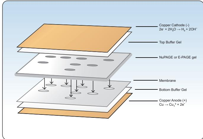
**Figure 7.** Gel/membrane sandwich with anode and cathode stacks
