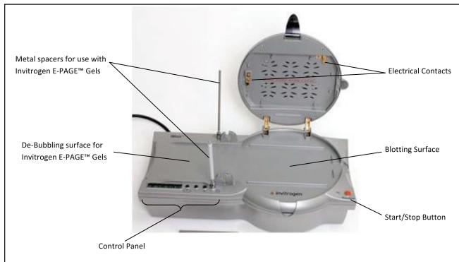
**Figure 6.** iBlot Gel Transfer Device
