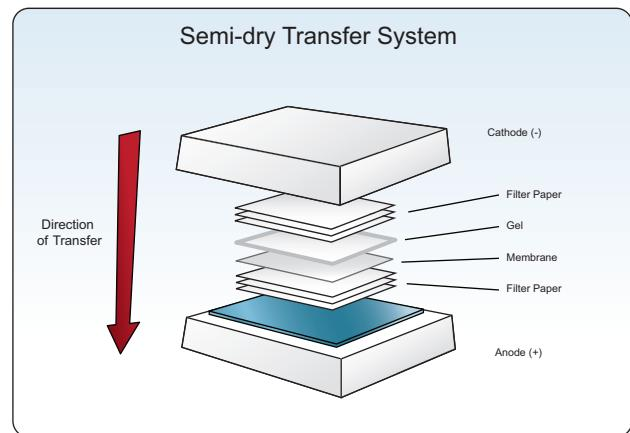
**Figure 4.** Diagram of semi-dry transfer setup.
