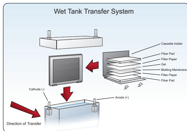
**Figure 2.** Diagram of Tank transfer setup.
