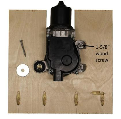
**Step 6:** Attach the motor to the motor mount plate. This design uses 1-5/8" wood screws. A large washer was used to anchor one of the corners, which had a much larger diameter anchor point.
