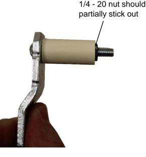
**Step 5:** Thread the second 1/4-20 nut partway onto the screw. Again you may have to file the corners. A lock nut is preferred, but if you don't have any apply an adhesive or plumbers tape to anchor it in place.
