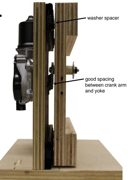
Side view of the finished assembly. Notice the good spacing between the yoke and the crank arm, which was created by adding the washer spacers.
