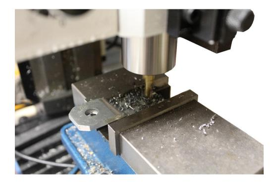
**Step 2:** Drill or machine out the post. Here we demonstrate a 1/4" diameter end-mill machining out the post.
