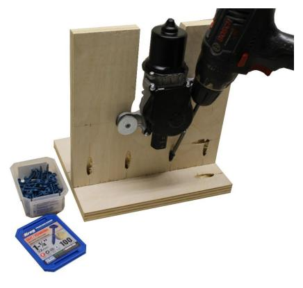
**Step 7:** When attaching the motor mount to the base plate, its needs to be about 7/8" (0.875 inches) offset from the center line. This offset is so that when the drawer glides are added, the yoke will move back and forth along the center line and push on the center of the Ambu Bag.
