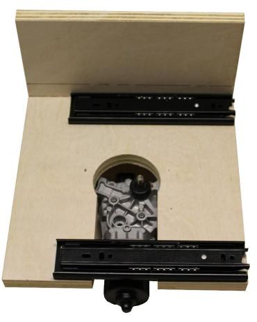
**Step 2:** Close drawer glides. **Note:** With 8" drawer glides, you will want the drawer glides to be flush with the rear of the motor mount plate to be able to screw into the narrow portion of the yoke.
