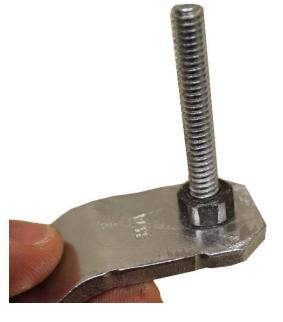
**Step 3:** Anchor the screw to the crank arm with the 1/4-20 nut. You may have to lightly file the corners of the nut to allow the nut to fit inside CPVC pipe. If you don't have access to lock nuts which would be preferred, use super glue, epoxy or even plumbers tape to minimize the potential for it to loosen.
