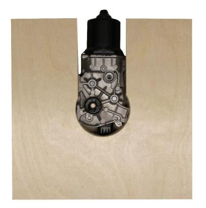
**Step 5:** Check the placement of the motor from both sides. The motor shaft doesn't need to be at the center of the board, but you want to confirm that the crank arm will not rub against the wood as is rotates. You may have to get creative and add spacers.
