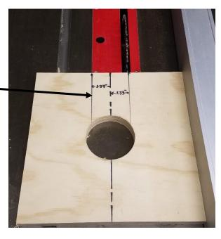
Step 4: Using a pockethole jig, drill pocket holes at the specified locations in the dimensioned drawing.
