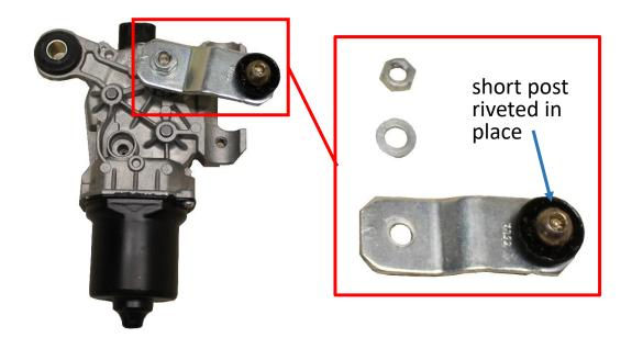
**Step 1:** Remove the crank arm from the motor shaft.
