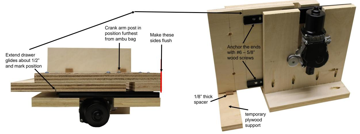
**Step 3:** Extend the drawer glides about 1/2" and then place the yoke on top with the back of the yoke flush with the back of the motor mount.
