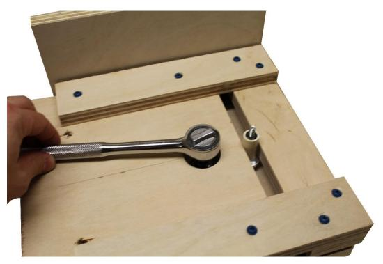
Step 8: Attach the crank arm to the motor shaft.
