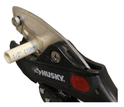
**Step 4:** Cut the CPVC pipe to length. This may very depending on your wiper motor, but for this design 1-1/4" to 1-3/8" is an acceptable length.
