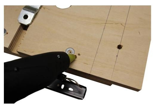
**Step 6:** For this design the yoke doesn't sit far enough away from the crank arm to keep it from rubbing on the inside surface of the yoke. To get around this, hot glue a 1/4-20 washer at as many of the anchor points of the inner drawer glide. This adds about 1/16" offset which is just enough clearance.
