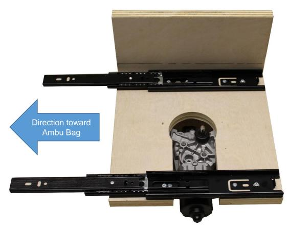
**Step 1:** Align the drawer glides along the top and bottom of the motor mount plate. Screw them in place with #6 - 5/8" long wood screws. This design can accommodate 8" and 10" long drawer glades. You can use longer glides, but you will have to make changes to parts of this design.
