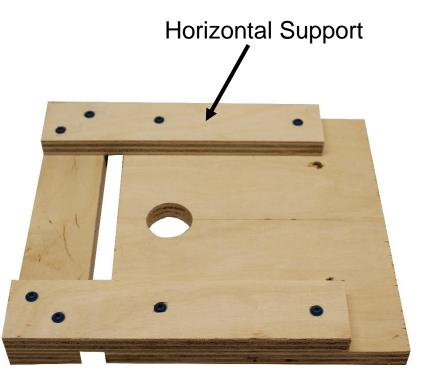
**Step 2:** Screw the horizontal supports in place with 1-1/4" wood screws and then remove the pipe and spacers.
