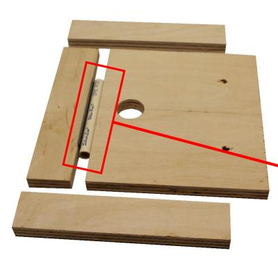
**Step 1:** The 1/2" CVPC will be rolling up and down the inside of the channel. Add a couple metal shims to give the tube clearance to roll.
