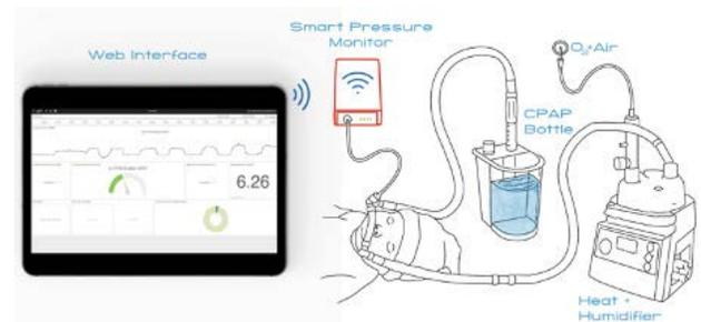
The diagram depicts a preexisting bCPAP circuit with the added smart pressure monitor. The device continuously reads the pressure of the bCPAP system and will alert nurses to abnormalities. The web interface and patient data display is accessed through an iPad or other computer.
