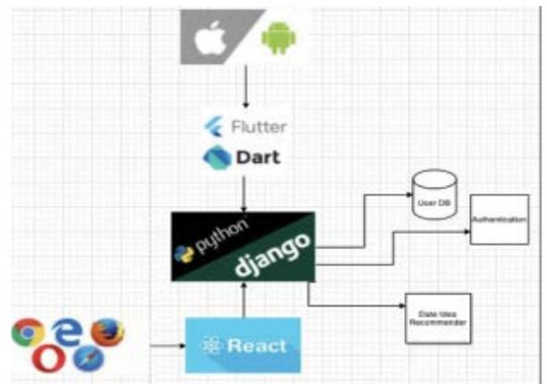
The Datr application consists of a web client, a mobile client, and a backend server that communicates with both. The backend server utilizes the Django Python framework and manages user authentication, data storage, and dating idea recommendations. The mobile and web applications are written utilizing Flutter/Dart and React, respectively.
