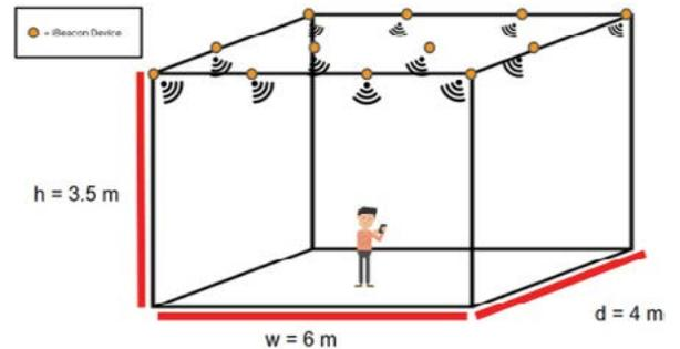
Our indoor positioning system uses BLE beacons installed in the ceiling to communicate with the Android device. Combining this input with the input from internal sensors on the phone allows the system to achieve the most accurate positioning capability.
