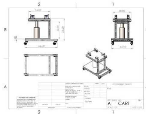
The stand for the chair includes a hydraulic lift to adjust the angle of the seat, wheels for easy mobility, and attachment points for the seat.
