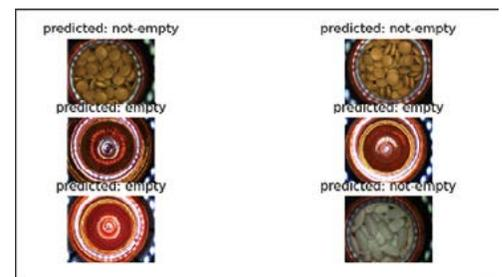
Results from a convolutional neural network trained to distinguish between empty vials and vials with pills inside. This model was trained as a binary classifier using transfer learning.
