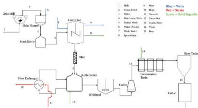
The process flow diagram demonstrates the layout of the brewery with the equipment and general ingredients needed to make the different brews.
