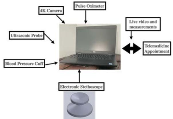
The telemedicine device includes an electronic stethoscope, ultrasonic probe, blood pressure cuff, 4K camera, and pulse oximeter.
