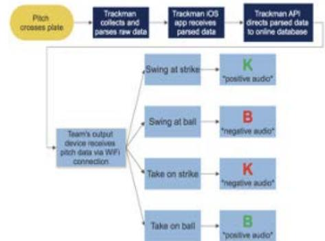
The system output gives customized visual and audio feedback to hitters based on pitch location and batter response.
