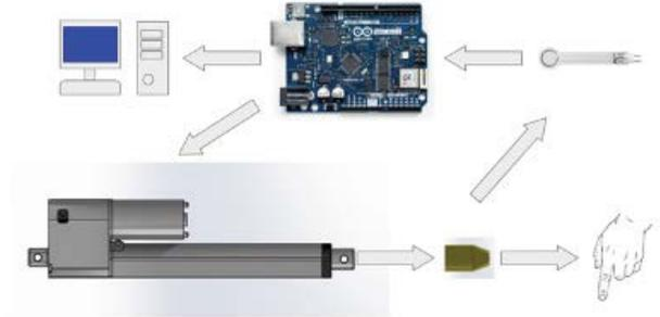
Pressure is exerted by the actuator on the pressure sensor and the finger through a rubber tip. The pressure sensor provides information to the computer and feedback to the actuator through the Arduino.
