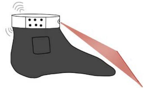
The system includes a Sensoria® sock and a cueing device that outputs visual, vibratory, and auditory signals for treatment of freezing of gait.
