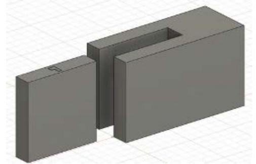
The device casing is comprised of two parts: a hollow enclosure for an RFID tag and a solid overlay that will connect to the hollow enclosure using an epoxy adhesive.
