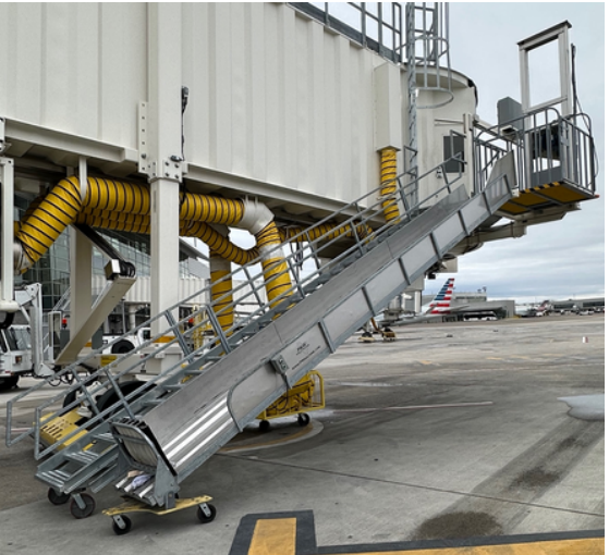
Luggage chute with elevator for safe wheelchair transport, a recent infrastructure addition missing at most jet bridges.
