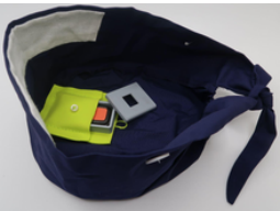
Above, Sample display of post-operative posture statistics. Right, One IMUs in protective casing in a scrub cap pocket.
