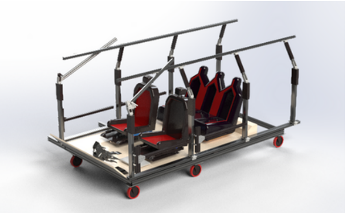
A full-scale reconfigurable interior buck designed to show a vehicle interior and cargo space. The system can adjust frame configuration, length and width of the vehicle, seating locations, and raise or lower the roof line. Wheels provide easier transportation and car-like appearance.
