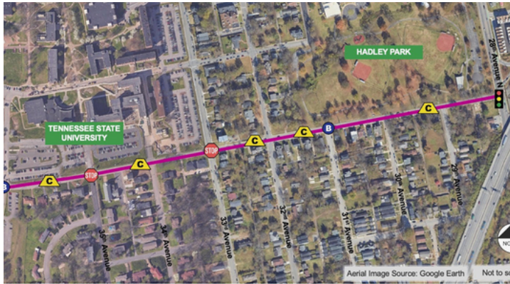
This traffic calming plan for Albion Street aims to enhance pedestrian safety and reduce vehicle speeds through the implementation of speed cushions (C), bulb-outs (B), and lane narrowing.
