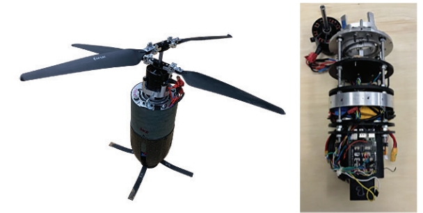
The coaxial drone, designated as the STEMnaut Atmospheric Independent Lander, is designed as a modifiable payload that jettisons from a rocket and is guided to touchdown through manual control.
