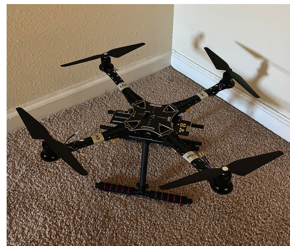
The low-cost UAV drone frame with motor, propeller, and component mount installed.
