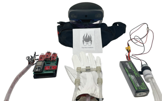
The thermal feedback device features thermoelectric modules for precise temperature simulation, a water-cooling system with a pump, Microsoft Hololens for AR experiences, and a custom PCB with a battery for seamless control and connectivity.
