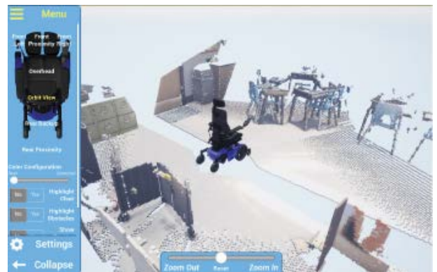
Permobil simulation software within the Unreal Engine 4 framework in which the group is designing the autonomous wheelchair additions and validating their project design. Depth cameras are placed strategically on the wheelchair to enable environmental awareness, and the ROS framework is used to process the depth camera data.
