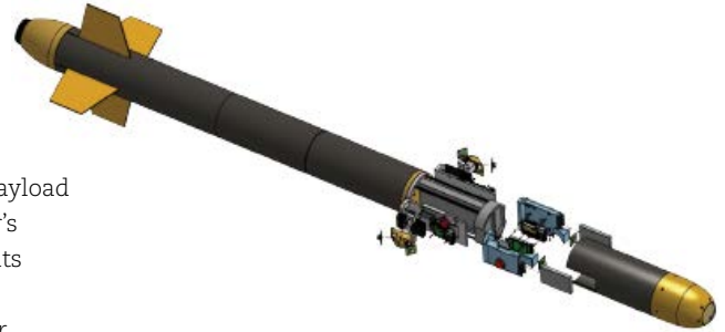
The 7-foot long launch vehicle with a modular and redundant payload system capable of autonomously identifying its landing location without the use of external systems.
