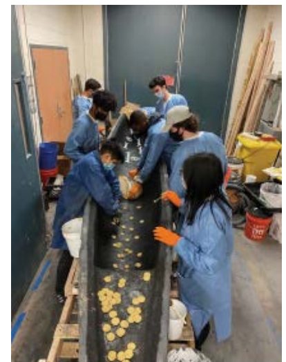
Vanderbilt Concrete Canoe team applies specially colored concrete to the mold to create the concrete canoe with the aesthetic design of Charon's Ferry .
