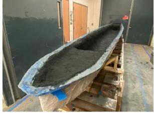
The concrete canoe in female mold curing with three concrete layers reinforced with two layers of basalt mesh.
