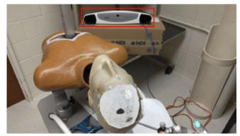
Using the Microsoft HoloLens 2 and an optical tracker (indicated by the red box), the virtual brain and tumor models of a craniotomy case were projected onto the physical head as if the user had X-Ray vision.
