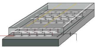
3D cross section of embedded thermoelectric generators in asphalt
