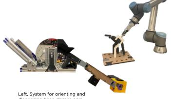
Left, System for orienting and dispensing hose clamps and (right) UR10e robotic arm and mechanism putting the hose clamps onto the hoses.
