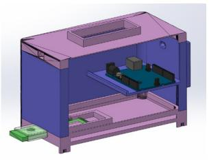
An assembly of the imaging box, including the sample tray and the mount for the Raspberry Pi camera.
