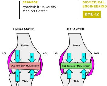
When the tibiofemoral gap is properly balanced, our device will measure equal tibiofemoral contact forces in the medial and lateral compartments.
