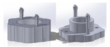
The illustration shows the end-vessel connection piece (left) and the side-vessel connection piece of the device (right). The holes and spikes on each piece lock to the corresponding features on the other piece.
