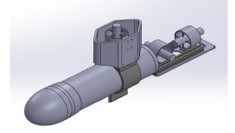
The streamlined hull design consists of a cylindrical base with a custom developed nose cone. Rear thrusters mounted to a plate provide a full plane of control, while a mounted dorsal thruster connected to the hull by a 3D printed collar provides the vehicle's depth control.
