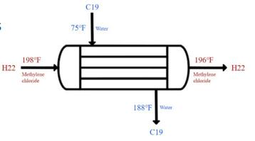
Addition of strategic heat networks to integrate hot and cold streams within the resin facility (such as the one shown) allows for multimillion-dollar annual operating cost savings.
