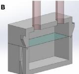
(A) shows the bioreactor with a transparent upper chamber, while (B) shows a section view of the bioreactor. The gray parts will be constructed using a bio-friendly resin printer. The red tubes are used for air intake and outtake (solenoids to control intake and outtake aren't shown). The green sheet between compartments is the rubber membrane.
