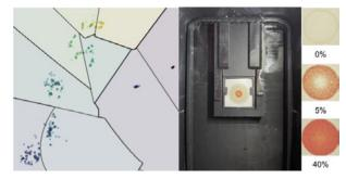
The algorithm discriminates between different percentages of sickled blood after taking a raw image and cropping out casing to leave only the blood sample.
