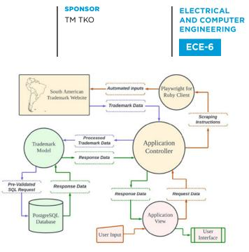
This diagram shows the flow of data through the application when a user requests the collection of new data. The Application View controls the user interface, accepting the user input and displaying results. The Application Controller controls interaction with each other component and processes the raw data. The Trademark Model handles all interaction with the database, allowing for database changes to be made without updates to the Application Controller or View.
