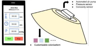
The vacuum bell includes a rechargeable lithium battery and automated pressure sensor, air pump, concavity measurement, and duration of use enabled through a Bluetooth Arduino.
