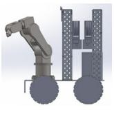
An autonomous robot on mecanum wheels that dispenses chips, identifies, organizes, and arranges objects, including battery container, autonomous arm, chip dispensers, solenoids, and camera.
