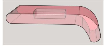
The product will facilitate holding a paintbrush onto a paint can without a clipping mechanism. The final design will include a way to open a paint can as well as connect itself magnetically to the steel wrap of a paintbrush and the rim of a paint can.
