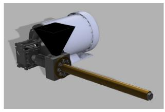
The assembly of key components of the PET extruder: motor, gearbox, coupler, flange, barrel, screw, die, and hopper.
