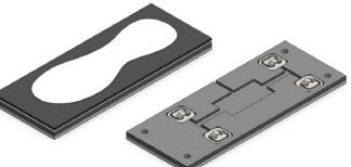
The footplate force sensor consists of a rectangular steel baseplate, a layer of 3D-printed plastic with cavities to hold the four load cells, a layer of aluminum to distribute the load, and a top layer of traction rubber.
