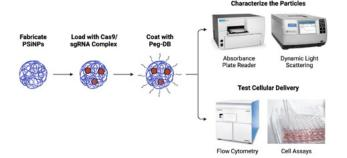
Schematic of the porous silicon nanoparticle (PSiNP) experimental workflow. First, PSiNPs are fabricated. Next, they are loaded with therapeutic cargo (Cas9/sgRNA Complex) and coated with a polymer stabilizer (Peg-DB). The finalized therapeutic nanoparticles are then characterized to evaluate loading properties and tested for efficacy and safety in vitro.
