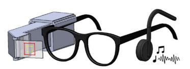
Integration of a custom heads-up display (HUD) with commercial bone conduction headphones that deliver improved auditory icons into a multisensory alarm system. Only one side of the headphones is shown for clarity.
