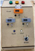
Left, concept drawing. Right, working prototype. The custom timing system includes a Raspberry Pi microcontroller, LCD display screens for the round display, work and rest periods, incrementing and decrementing timing controls for each display, LED status lights for quick activity indicators, a sound system, an emergency pause/stop button and an audio output sound selection control.
