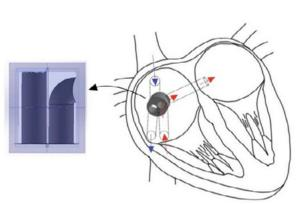
Our 3D-printed cannula cap allows for a single external incision to direct blood through two cannulas (dotted lines). One cannula brings deoxygenated blood (blue arrows) to an extracorporeal membrane oxygenation (ECMO) pump from the right atrium. while the other cannula redirects oxygenated blood (red arrow) across the atrial septum into the left atrium.
