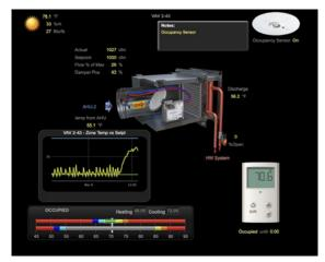
Metasys Automated Control software interface is used to interact with, monitor, and control environmental conditions on campus through existing HVAC infrastructure.
