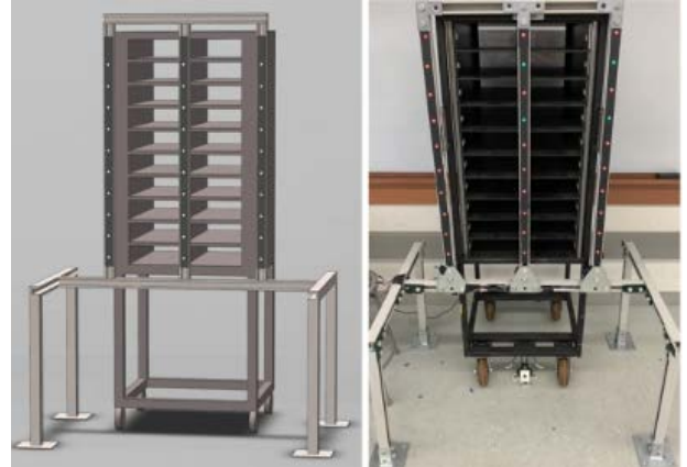
The CAD model (left) has three columns of lights and is used with carts that have two columns of bins. The prototype (right) is shown in front of an existing cart model. The green lights direct users filling the bins where to load the next parts.
