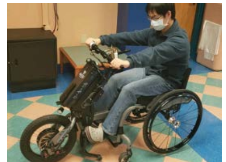
Prototype for handlebar and new control interface on a BATEC electric front-attachment, with wheelchair and user
