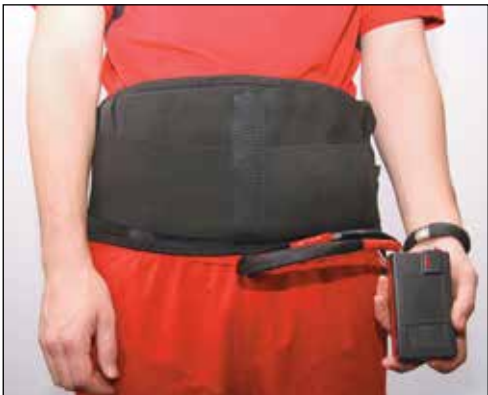
The prototype can detect a change in sitting or standing and inflate or deflate the belt automatically.
