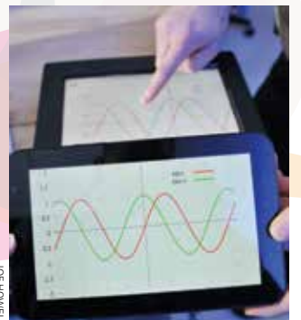
A haptic tablet translates the teacher's graphic to touch.
