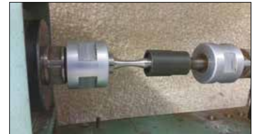
Specimen loaded for fatigue testing.
