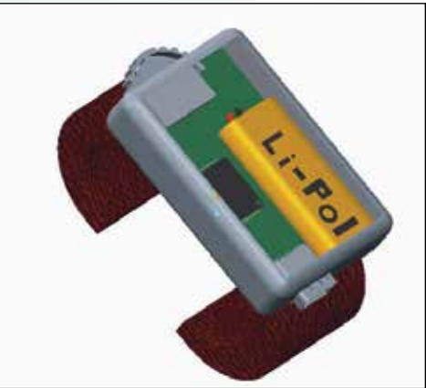
The CompleteControl unit including switch, wireless module, battery and charging port.
