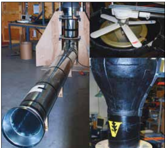
(Clockwise from left) Intake duct and inline fan; Wind turbine with ogive; Redesigned exhaust stack funnel.
