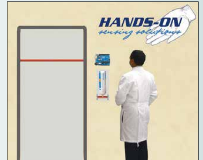
The integrated sensing system above tracks doorway entry and hand sanitization in order to record and improve hand hygiene compliance.
