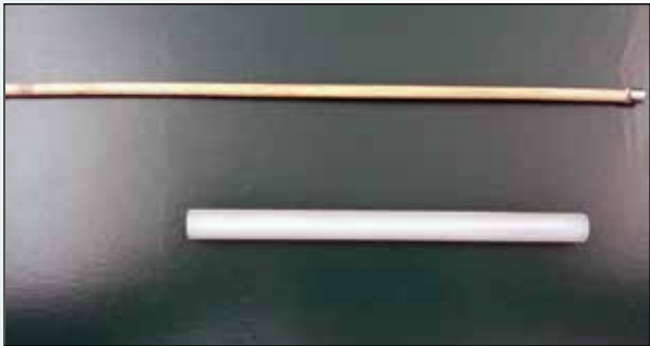
The Extractionator tube with the magnetic field applicator.
