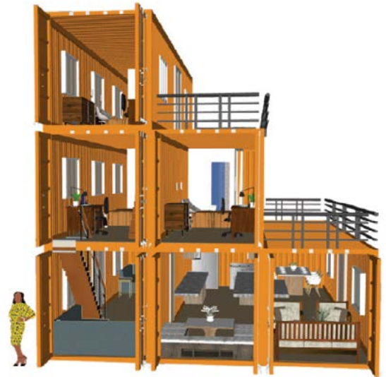
3D model of a residential unit built using six 40-foot shipping containers with bedrooms, bathrooms, kitchen, dining, and living space
