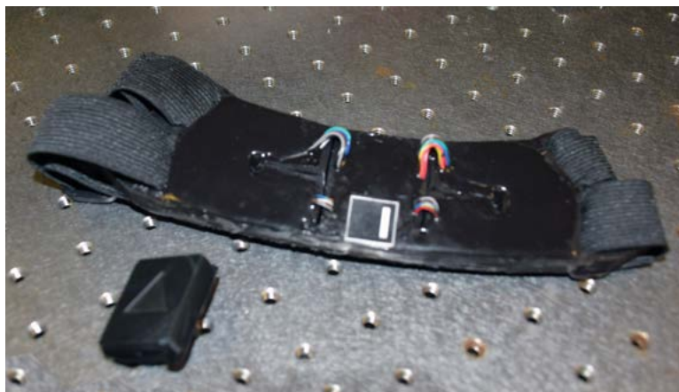
The DIY headband device weighs about 5 ounces, including its battery pack. It can be assembled with easily available components for a cost of less than $250, compared to commercial devices that can cost $10,000 or more.
