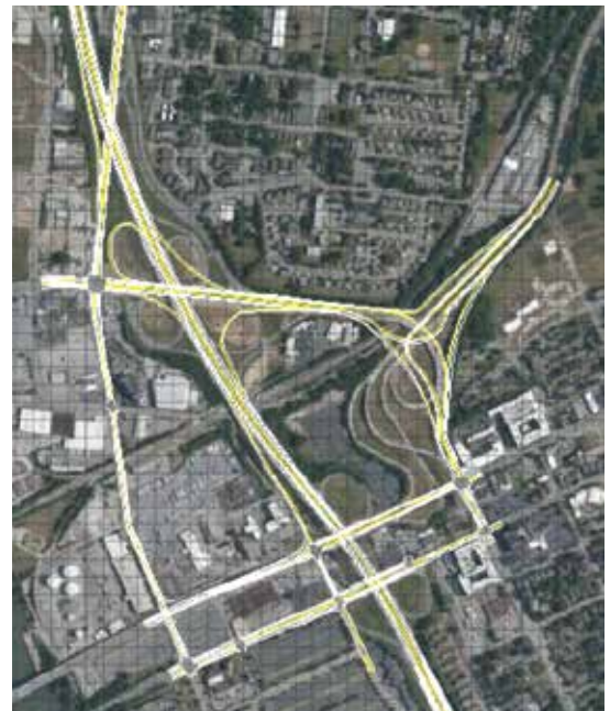
A preliminary design for Spaghetti Junction is superimposed on the current layout of the project area.
