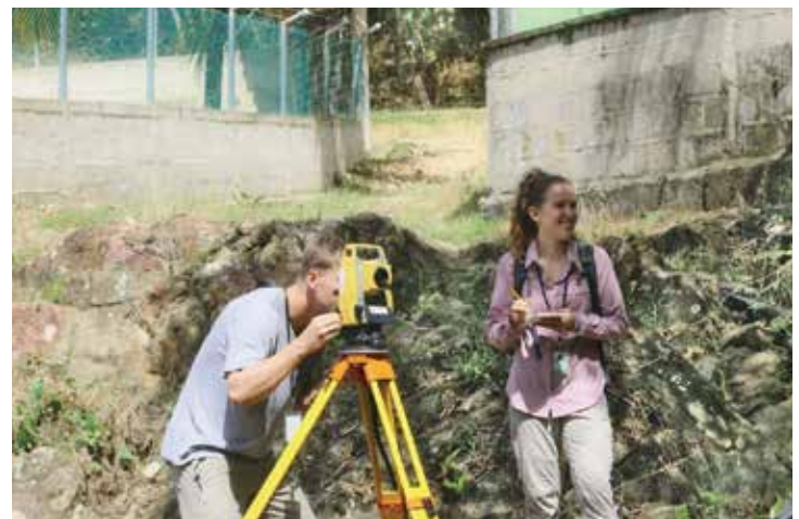
Team members Nathan and Caroline survey the riverbed in order to draw a topographic map and complete a hydrologic analysis for the proposed bridge in Bacadillas, Honduras.
