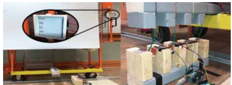
Left, Prototype on a sample kit cart running its path in the factory. Right, Brushes and contacts meet to transfer power and data to update the e-paper display.
