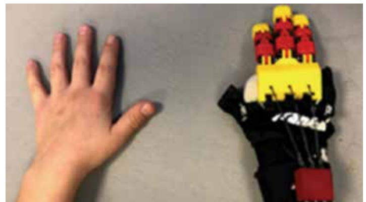
Gage wears the first prosthetic prototype. The hand is designed, built and tested to be a custom wrist-actuated prosthetic for a very active youngster.
