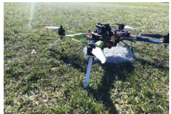
Pictured above is one of two autonomous UAVs that will deploy from a rocket payload bay and complete a collaborative search-and-deploy mission through a self-contained navigation system.
