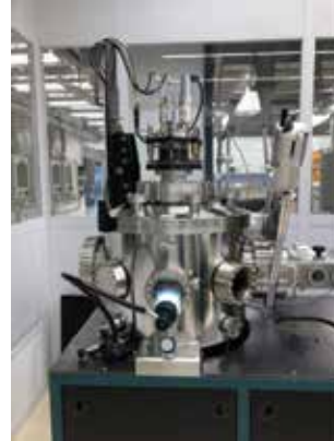
Left, A thin film deposition system that coated the prototypes. Right, A prototype glass sample coated with a triple bi-layer of aluminum oxide with titanium dioxide.
