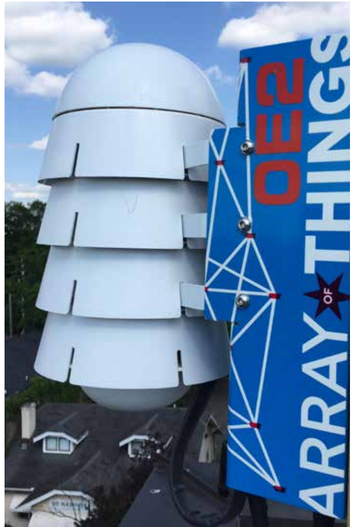
Sensor nodes collect air quality and transportation data across the Vanderbilt campus. The arrays are about 18 inches tall, 14 inches deep and 9 inches wide.
