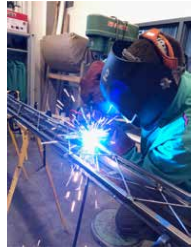
Steel Bridge team members cut, welded and/or drilled each individual part and piece of the steel bridge.
