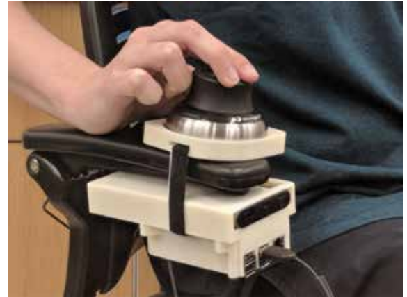
The device attached to the arm of a wheelchair allows a user to wirelessly control a robot arm and its mobile base with a 3D mouse.
