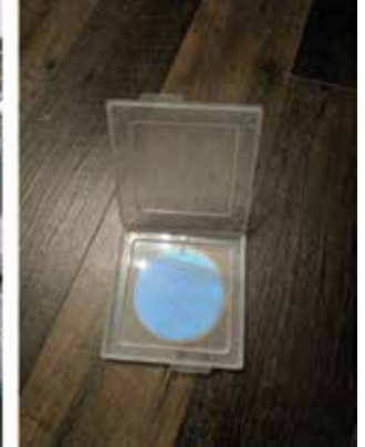
Left, A thin film deposition system that coated the prototypes. Right, A prototype glass sample coated with a triple bi-layer of aluminum oxide with titanium dioxide.
