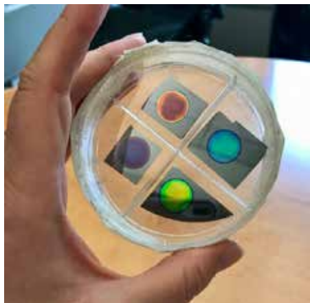
Silicon chips coated in porous, nanoscale films could be used with an iPhone and future app to quickly detect infection and water potability with a drop or two of the liquid.
