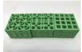
Left, 3D printed syringe prototype. Right, three plant growth substrates 3D printed from starch-based materials.
