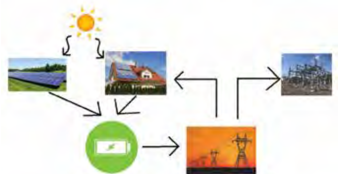
Solar energy is captured via rooftop solar panels and community solar gardens and stored in a central battery unit. Stored power can be redistributed to Sterling Ranch homes or other needs within Xcel's full grid.
