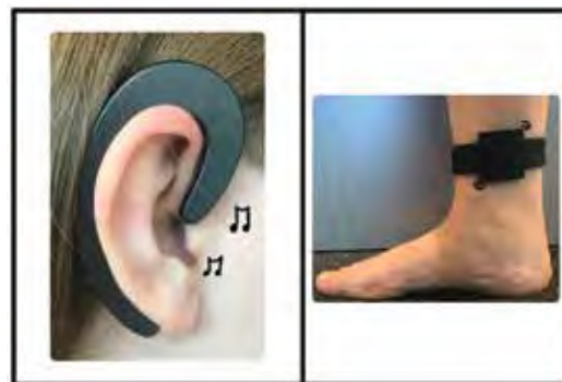
The multisensory alarm system utilizes both an auditory stimulus from sonification of physiologic data and a haptic (vibrotactile) stimulus on the clinician's ankle.
