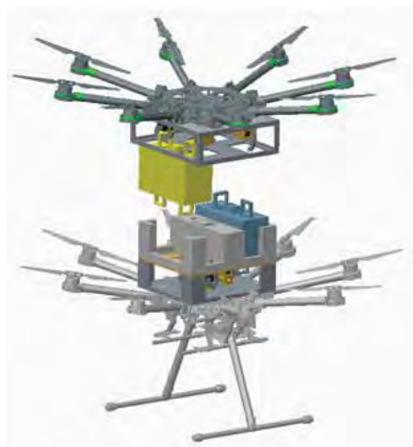
A payload octocopter (top) has its battery swapped by a refueling drone (bottom) to demonstrate the Touch-n-Go™ mechanism.
