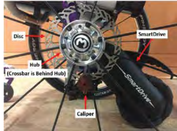
An automated disc brake system for a manual wheelchair used in conjunction with MAX Mobility's SmartDrive
