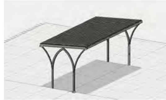
Curved arches that pay homage to the adjacent Buttrick Hall are featured in the structural steel design.
