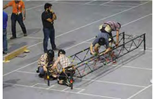
The steel bridge is a 1:10 model of the imagined final bridge. Eighty separable, custom-fabricated pieces comprise the 18-foot span.
