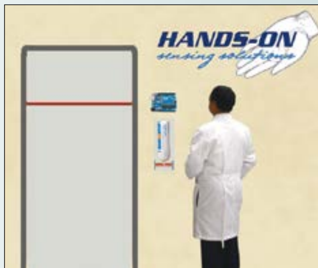
The integrated sensing system above tracks doorway entry and hand sanitization in order to record and improve hand hygiene compliance.
