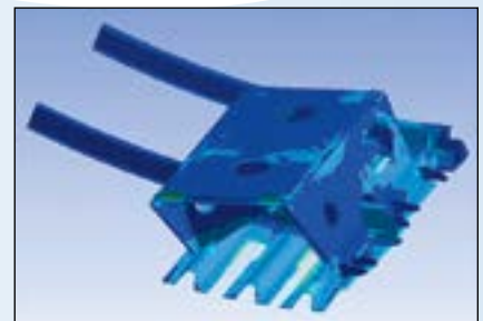
Existing Fan Support Bracket Stress Analysis.
