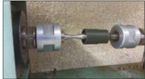
Specimen loaded for fatigue testing.
