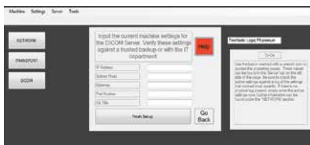
Example of troubleshooting the settings within the Network layer of a GE LOGIQ Ultrasound machine.
