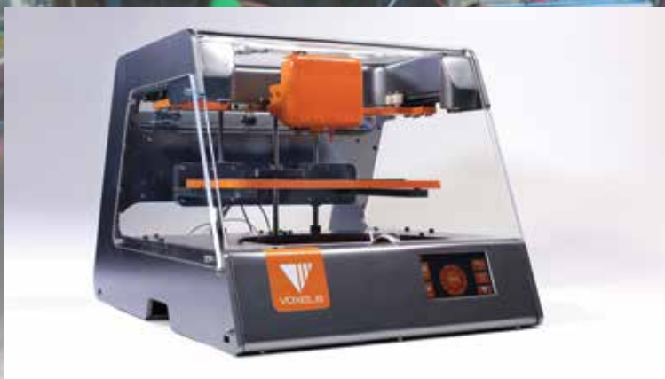
Alumnus Jack Minardi's new Voxel8 3D printer can make custom circuit boards in 30 minutes. It also produced this working UAV.
