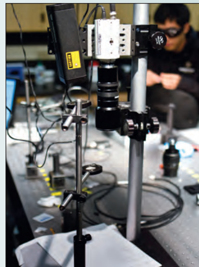
An image of preliminary laboratory validation with all optical components (laser, CCD camera) visible.
