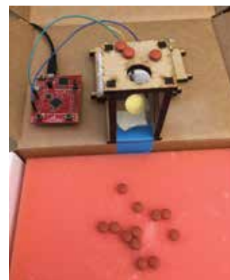
An early prototype of our sensor analyzes the sound that pills make as they drop onto a glass plate.
