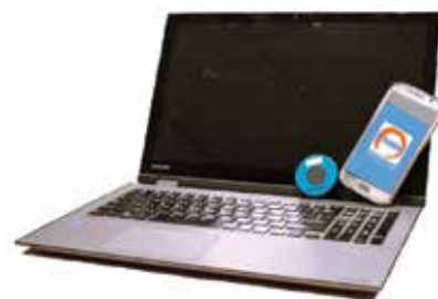
Devices utilized in the Dr. Roundabout System – beacon, smartphone with app, and computer
