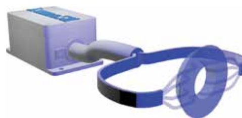
3D rendering of LumaSil, a low-level light therapy device to aid diabetic foot ulcer healing. Light generated in an external module on the cast is delivered to the wound via fiber optic cables embedded in a silicone halo.
