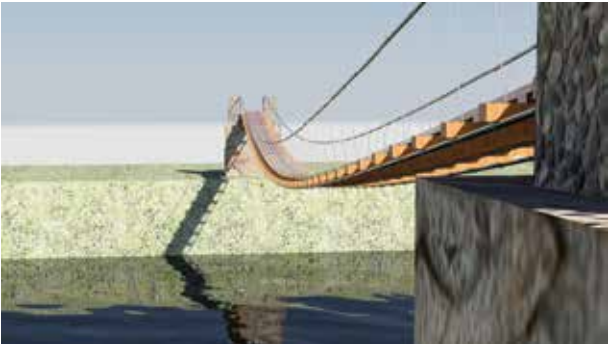
3D rendering of the student-designed 165-foot-long suspended pedestrian bridge over the Rio Grande in Honduras.
