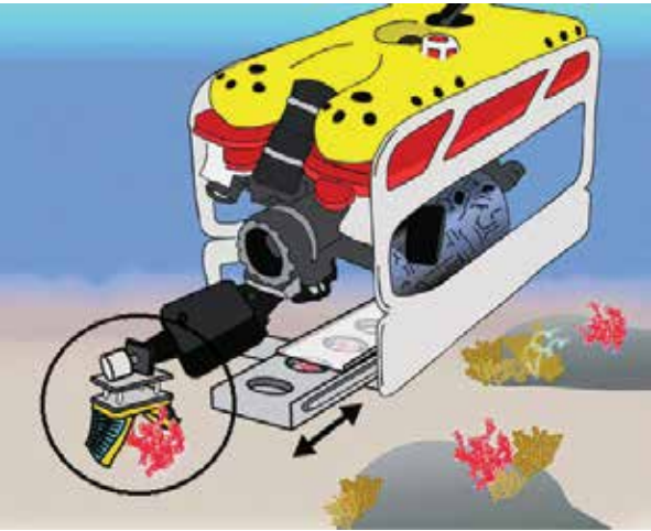
Illustration of a remotely operated vehicle (ROV) collecting samples from the sea floor. Circled is the portion that our team has redesigned.
