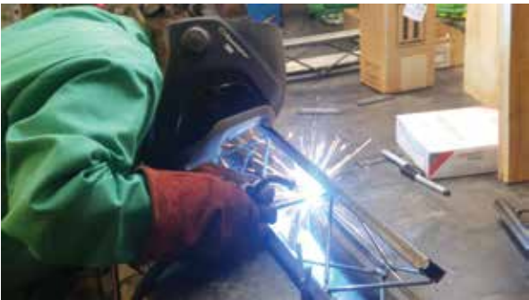
A member of the Vanderbilt Steel Bridge Team MIG welds steel lacing between three foot tube sections for the lower chord of the bridge.
