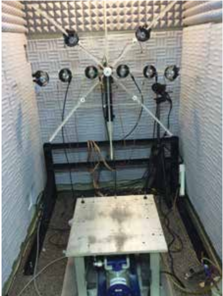
The LED bank will be attached to the speaker apparatus currently used in the Ramachandran Lab, shown above. By creating an LED bank that covers the frontal visual field of a monkey, we hope to aid researchers in the Vanderbilt Department of Hearing and Speech in their study of sensory integration.
