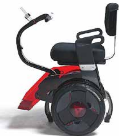
The self-balancing NINO Robotics wheelchair.
