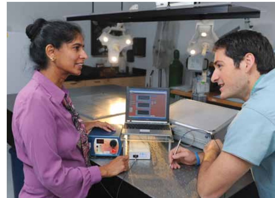
Professor Anita Mahadevan-Jansen sets up a system for the non-invasive detection of the parathyroid gland using near infrared autofluorescence.
