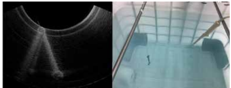
Ultrasound was used to produce high quality images of various tools submerged in water at distances of a few centimeters up to a meter. Such images will allow divers to "see" in their zero visibility environment.
