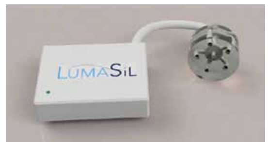
3-D design of LumaSil, a low-level light therapy device to aid diabetic foot ulcer healing by reducing the presence of infectious and antibiotic-resistant agents. Light generated in an external module on the cast is delivered to the wound via LEDs in a circular silicon design.
