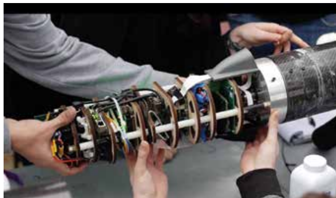
The fully assembled VADL real-time target detection payload attached to the rocket body prior to launch
