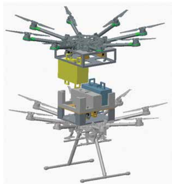
A payload octocopter (top) has its battery swapped by a refueling drone (bottom) to demonstrate the Touch-n-Go™ mechanism.
