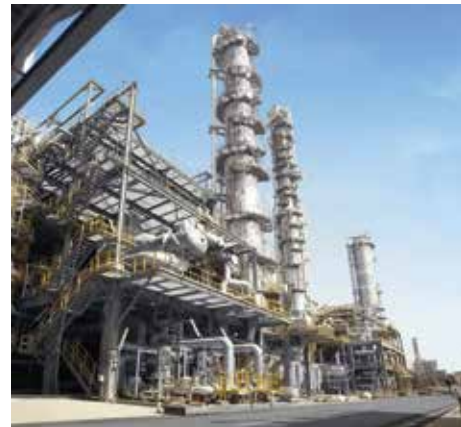
Distillation columns are common in chemical plants and they require a lot of utilities. Heat and mass integration could heavily reduce their utility consumption.
