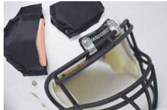
A frontal cross-section of a football helmet provided by the Vanderbilt University football program. A thin layer of shock absorbing material is enclosed inside of an air-tight, water-tight packet that is snapped to the traditional helmet shell.
