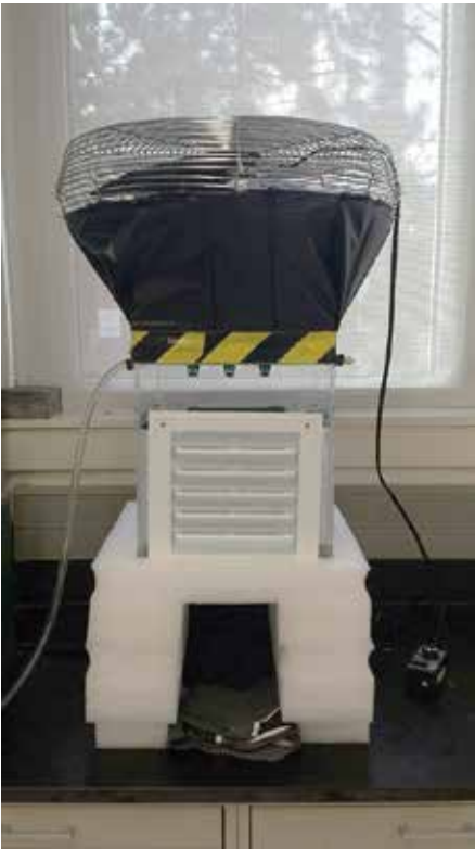
Cooling tower prototype used to find cooling results through different fan speed operations and atmospheric conditions.
