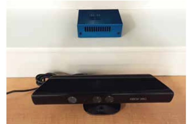
An Xbox Kinect and a Minnowboard within its case. The single board computer (SBC) operates the Kinect within NICU rooms to monitor infant interactions.
