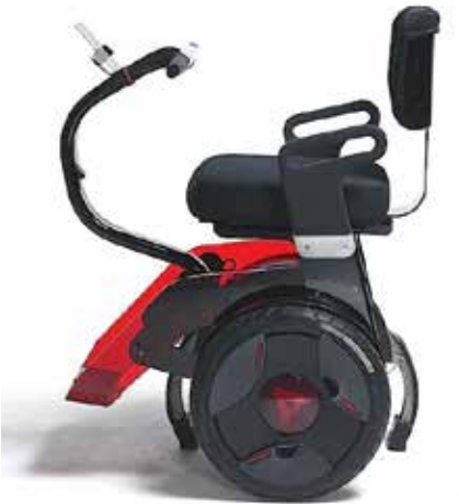
The self-balancing NINO Robotics wheelchair.
