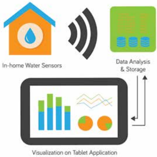
In-home water sensors feed meter readings to data analysis software, which communicates with the in-home tablet application to display a visual analysis of the home's water consumption to residents.
