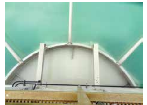
This is a reactor clarifier for use in brine treatment within a chlor-alkali process.
