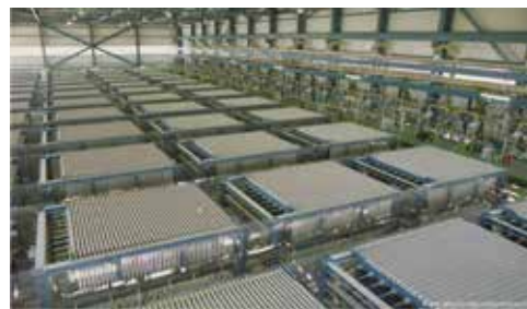
A chlor-alkali electrolysis process we aim to improve by recycling reagents that leave in the waste stream.
