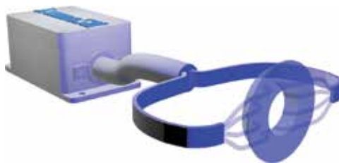
3D rendering of LumaSil, a low-level light therapy device to aid diabetic foot ulcer healing. Light generated in an external module on the cast is delivered to the wound via fiber optic cables embedded in a silicone halo.
