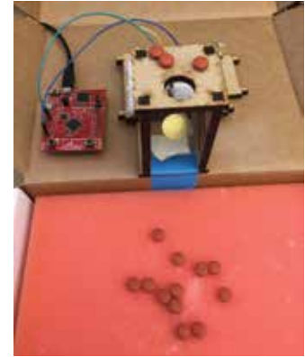
An early prototype of our sensor analyzes the sound that pills make as they drop onto a glass plate.
