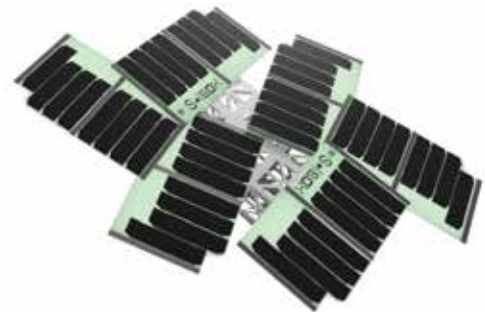
Depiction of CubeSat system with solar panels fully deployed
