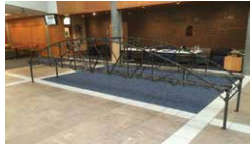
The 1:10 model bridge weighs 285 pounds, spans 20 feet, and stands 5 feet tall.
