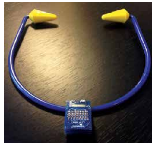
A photodiode placed within the ear cap canal will receive IR, relay that information to the Arduino compatible board, and transmit the temperature data via Bluetooth to a computer.
