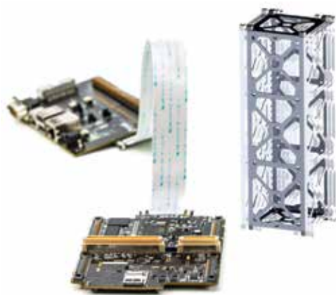
CubeSat satellite system bus and computer model of a vibrating frame
