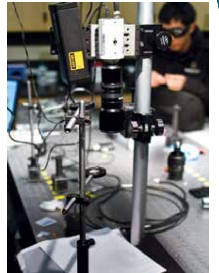
An image of preliminary laboratory validation with all optical components (laser, CCD camera) visible.
