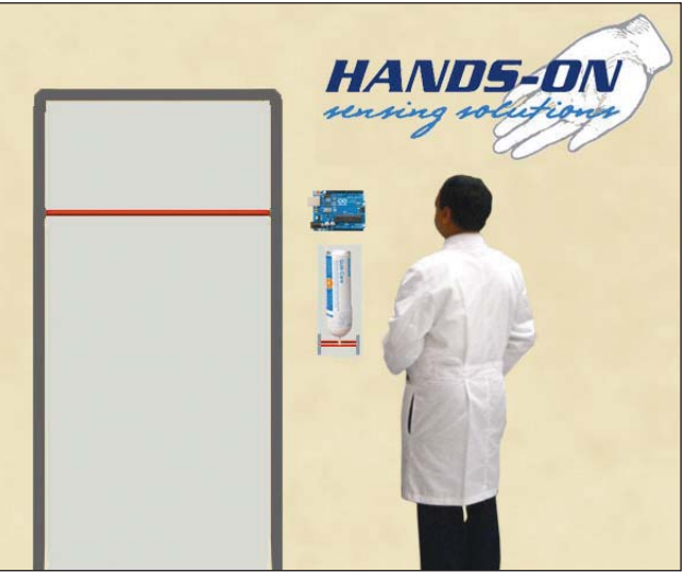
The integrated sensing system above tracks doorway entry and hand sanitization in order to record and improve hand hygiene compliance.
