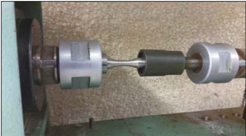
Specimen loaded for fatigue testing.
