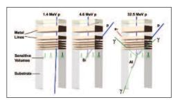
Events causing single event upsets for 1.4, 4.6, and 32.5 MeV incident protons. The material dimensions have been reduced for illustration purposes
