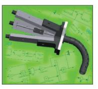
Since the robot enters through the natural opening of the oral cavity, the patient will not be left with visible scars following the operation. The function of this tendon-actuated channel is twofold: it assists surgeons to accurately and safely deploy surgical tools into the upper airways, and it provides the patient the option of a more comfortable and less invasive surgery.
