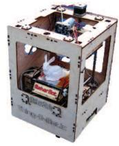
The Thing-O-Matic® 3D Printer comes in a do-it-yourself kit. It can print in plastic almost any design within a 96x108x115mm build volume.
