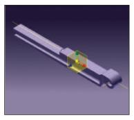
The new clamp design uses a round, inflatable surface to occlude the vessel.
