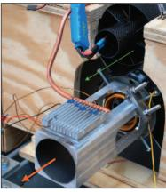
Rocket flight experimental simulation setup showing scaled model of TEG engine, J90 rocket motor, cryogenic injection system and high-speed VASA fan for establishing parity between rocket and airplane flight.
