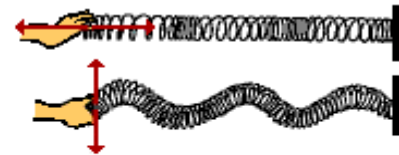
Slinky waves can be made by vibrating the first coil back and forth in either a horizontal or a vertical direction.
