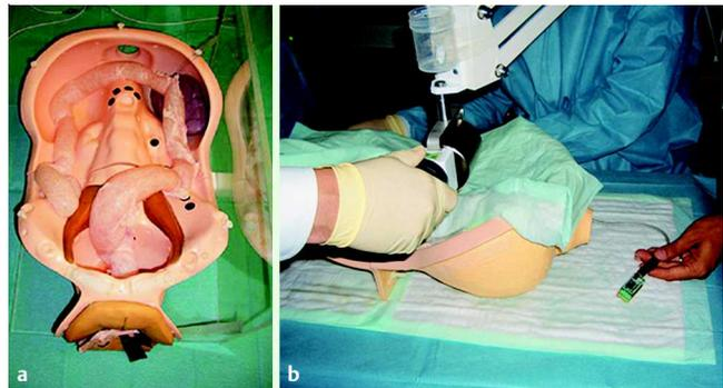
**Fig. 2** a Lower gastrointestinal (LGI) tract phantom before the experiment. b LGI phantom during the experiment, with the external permanent magnet and the transceiver clearly visible.
